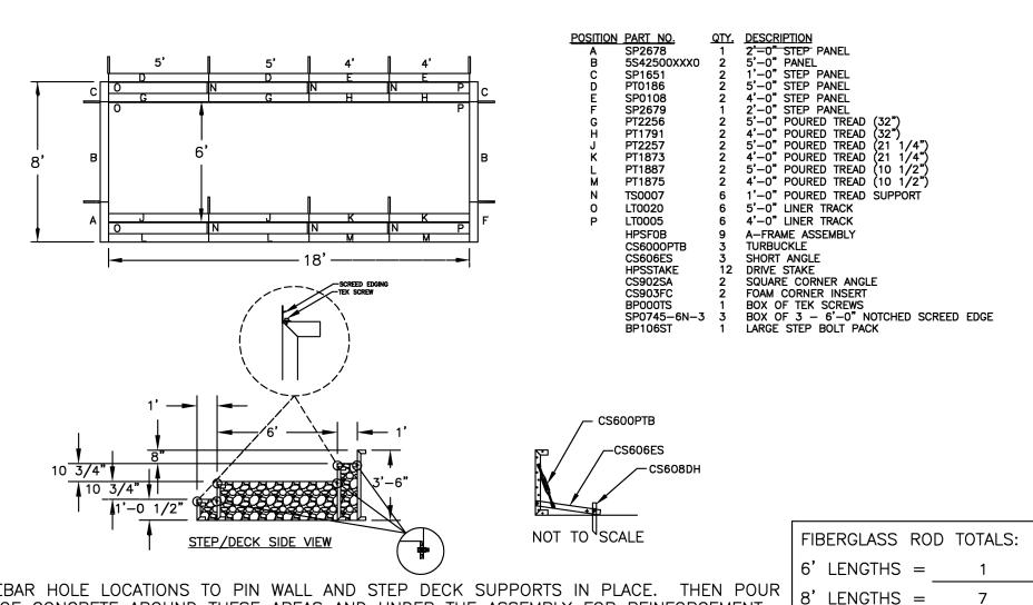
USE REBAR HOLE LOCATIONS TO PIN WALL AND STEP DECK SUPPORTS IN PLACE. 4"-6" OF CONCRETE AROUND THESE AREAS AND UNDER THE ASSEMBLY FOR REINFORCEMENT
